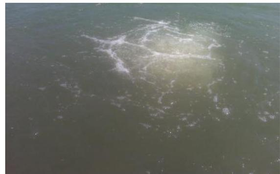
Photo of a diffuser boil created from a single diffuser head. Photo courtesy of LEI.
